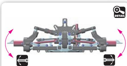
When the bars are set, verify that both sides move at the same time. If they do, the bars are set up correctly. If not, make sure that both downstops are the same and that the bar wire is flat.
